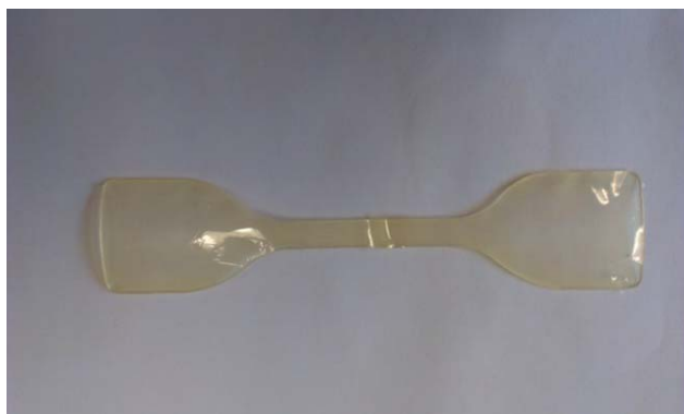
Figure 3. Tensile test specimen of P13 . [Color figure can be viewed in the online issue, which is available at wileyonlinelibrary.com .]
