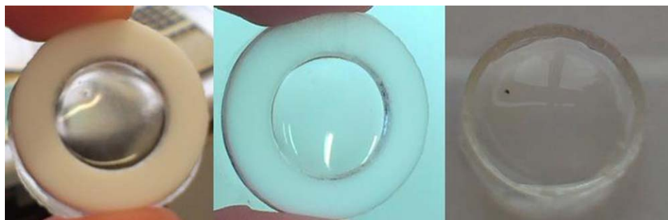
Figure 1. Polymer films of PI obtained via photo-polymerization. [Color figure can be viewed in the online issue, which is available at wileyonlinelibrary.com.]
